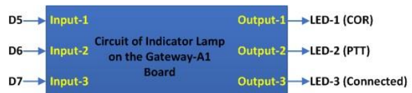
Figure 15. The connection of the indicator lamp circuit
