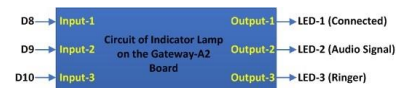
Figure 21. The Connection Pins in Circuit of Indicator Lamp on the Gateway-A2 Board
